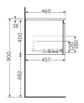
Dimensions: All dimensions in mm. Tolerance of vitreous china & fireclay items:  $\pm$  5% for below 200mm and  $\pm$  3% for above 200mm; for all other items tolerance  $\pm$  1%. Note: Due to a continuing development program to improve design and performance, the manufacturer reserves all rights to vary specifications without prior information. Please note accessories are for photographic use only.
