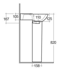
Dimensions: All dimensions in mm tolerance  $\pm 5\%$  for below 200mm and  $\pm 3\%$  for above 200mm. Note: Due to a continuing development programme to improve design and performance, the manufacturer reserves all rights to vary specifications without prior information.
