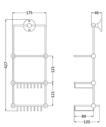
All Dimensions are in millimetres. The information contained on this page was correct at date of issue. Fitting dimensions are provided as a guide only. Some variation may occur due to manufacturing tolerances. We pursue a policy of continuing improvement in design and performance of our products and so reserve the right to change specifications without prior notice.
