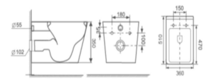
Notes: The center distance of the mounting screw hole is 180mm
